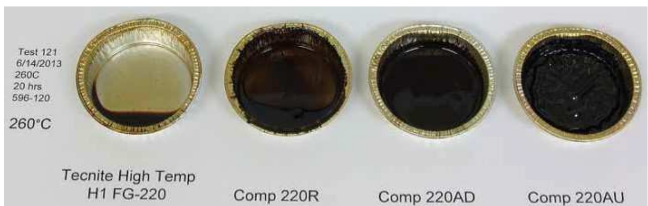
Figure 1 – Fewer deposits on metal as Tecnite remains liquid even after long exposure to temperatures up to 260°C. Less time devoted to cleaning chains result in substantial cost savings.
