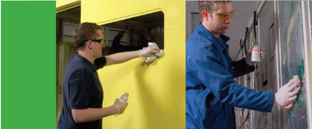
Far left: Apply BETAWIPE with a continuous movement to clean and activate surfaces as part of a complete adhesive system.
