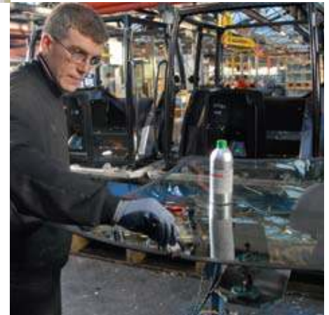
Above: Used as part of a complete glass bonding system, BETAPRIME is also used as an adhesion promoter on body surfaces in conjunction with BETAMATE™ structural adhesives.
