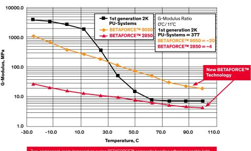
Two-component, room-temperature curing BETAFORCE™ composite bonding adhesives enable light-weighting and dissimilar material bonding. The adhesives are optimized to retain strength and rigidity at elevated temperatures, providing industry-leading temperature stability for customer applications.
