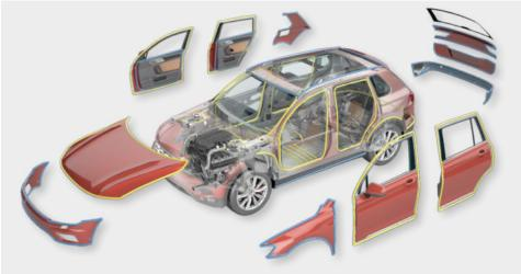
BETAFORCE™ is an ideal choice for joining carbon fiber and glass fiber composites and other dissimilar materials in a variety of lightweight designs, including modular assemblies. It can be used to bond coated metals like steel to aluminum, carbon fiber panels to steel or aluminum and sheet molding compound (SMC) to aluminum.
