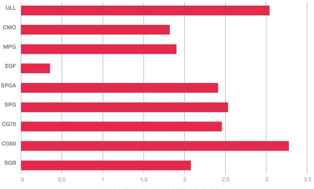
WEAR RESULT AT 100kgf PRESSURE LOAD (mm)
