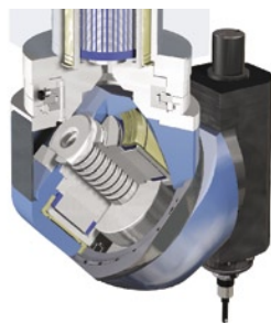
Asse A 45° universale • 15 kW/74 Nm mass./ 24.000 giri min mass.
