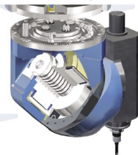
Asse A 45° universale • 20 kW/130 Nm mass./ 18.000 giri min mass.
