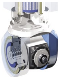
Asse A Forcella (S8) • 8 kW/35 Nm mass./ 24.000 giri min mass.
