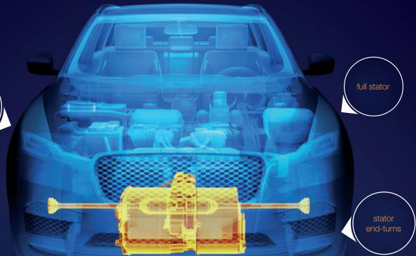
Araldite<sup>®</sup> encapsulants and impregnation resins for e-motor improve heat dissipation and extend lifetime Araldite<sup>®</sup> encapsulants and epoxy impregnation resins increase performance of rotor, full stator and stator end-turns
