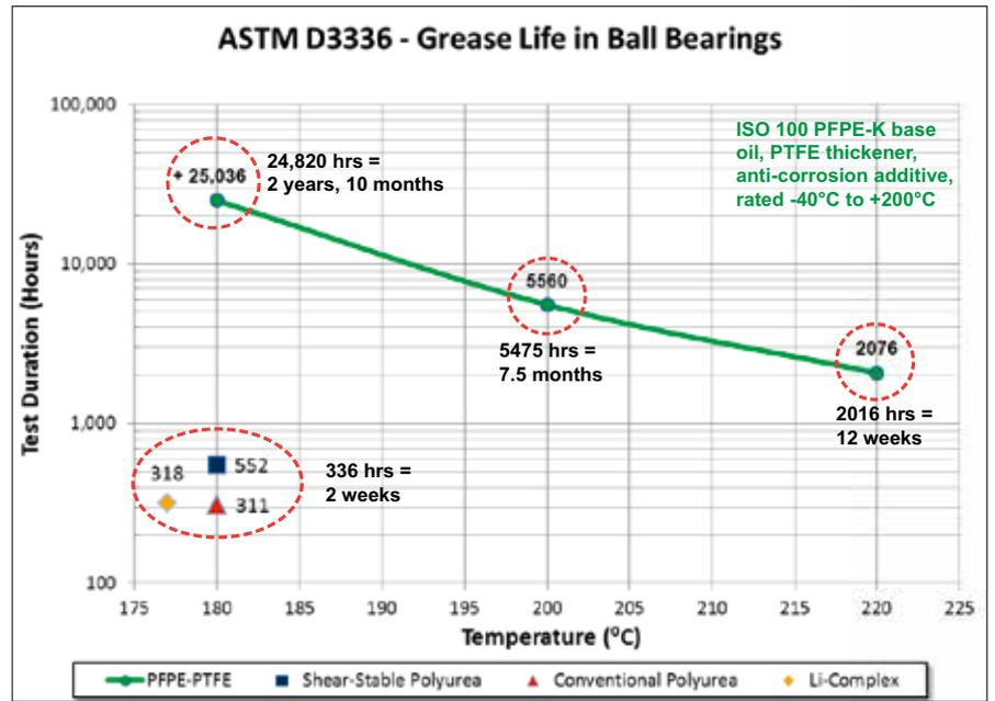
Results of the ASTM D-3336 testing on a Krytox™ grease compared against standard electric motor bearing greases. They are for a lightly loaded 6204 bearing at 10,000 rpm. The test cycle was 20 hours on and 4 hours off.
